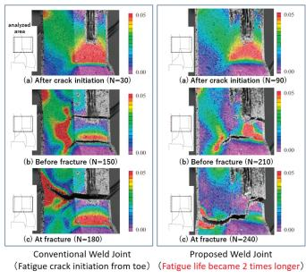
Fig 2 Max. strain distribution measured by DIC (Low-cycle fatigue test of weld joint)
