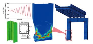
Fig 1 Digital Twin of Bridge pier (Cyclic elasto-plasticity FEM simulation)
