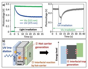
Fig. 2. a) UV-induced photovoltage drop and recovery. b) The mechanism of WDPE behavior
