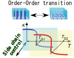
Fig 1 Tuning the switching temperature in thermal switch using the order-order transition in liquid crystalline block copolymer. Choosing the type of mesogens in the side chain in liquid crystal part modulates the switching temperature.
