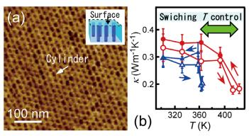
Fig 2 (a) Atomic force microscope image of the surface of block copolymer including cylinder (low temperature phase).
