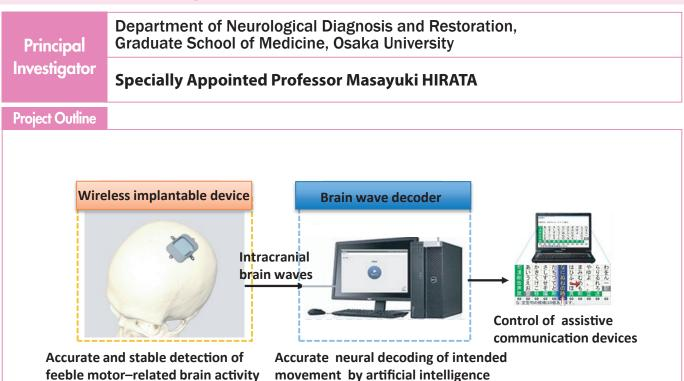
A brain-machine interface (BMI) is a technology used to read the contents of motions and communication from brain signals and to control robot arms and communication devices. This is expected as a technology to restore the impaired functions of disable people. In this project, we aim to perform a clinical trial of an implantable BMI device that records accurate brain waves using brain surface electrodes and to license it to a medical company.
