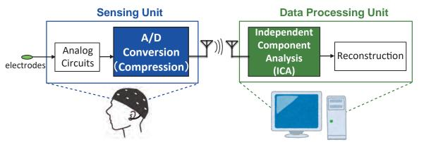
Compressed sensing allows sampling while compressing the signal, reducing the amount of information handled by the circuit, and thus enabling low power consumption of the circuit. This leads to a smaller battery size and longer operation time. However, general compressed sensing, has the problem of being vulnerable to disturbances, which reduces the accuracy of reconstruction.
