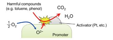
Figure 1. Schematic illustration of decomposition of harmful organic compounds using oxygen supply from the promoter toward the activator.
