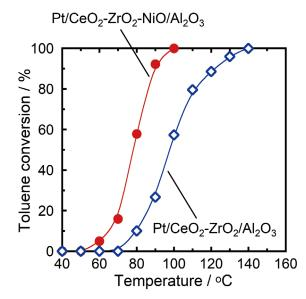
Figure 2. Temperature dependence of toluene conversion over Pt/CeO\_2-ZrO\_2-NiO/ Al\_2O\_3 and Pt/CeO\_2-ZrO\_2/Al\_2O\_3.
