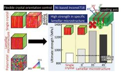
Figure 2. Flexible control of crystallographic texture achieved via metal 3D printer, and unusual strengthening by forming a specific lamellar structure (example of Inconel 718). Further strengthening is achieved by changing the resistance to slip deformation at the layer interface by changing the loading axis.
