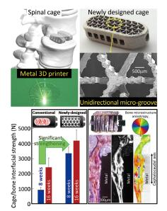
Figure 1. Titanium alloy spinal cage with a micro-groove structure based on the precise shape control capability of a metal 3D printer. The micro-groove structure induces mechanically integrated high quality bone, resulting in a significant increase in strength at the initial implantation period compared to conventional cages.
