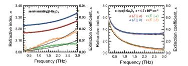
Refractive index spectra for wide bandgap semiconductor of  $\beta\text{-}\mathsf{Ga}_2\mathrm{O}_3$  in Terahertz range
