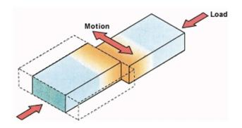
Fig. Schematic drawing of LFW
