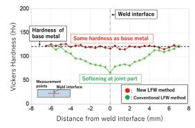
Fig. Hardness distribution of Al6061-T6 joints
