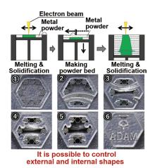
Fig. 1 A schematic drawing of EB-PBF process. It is possible to control internal shape of 3D products by adding layer-on-layer of material.
