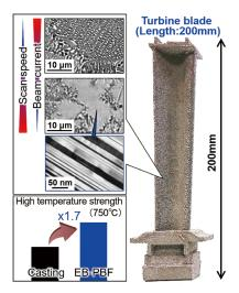
Fig. 2 It is possible to control microstructure of TiAl alloys by EB-PBF. A nano-scaled lavered microstructure can be obtained through a unique phase transformation. The strength of the allovs with the nano-scaled lavered microstructure is 1.7 times higher than that of casting alloys.
