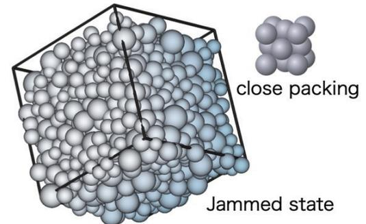
Fig. 1 Hard-sphere glass at a high density close to jamming density
